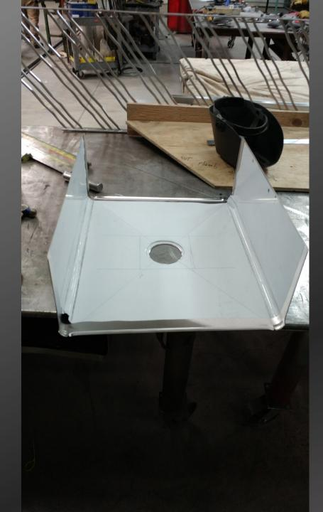
Forming the sing bowl is up next. The radius edges of the bottom and sides are starting to take shape
