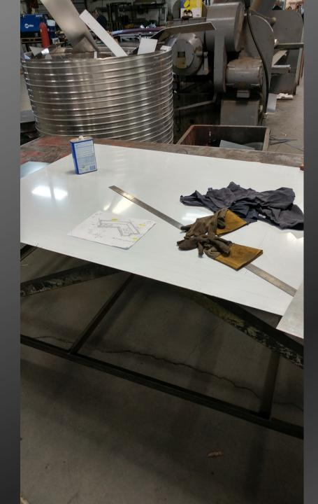
The process is underway with a blank sheet of stainless steel and the layout drawing
