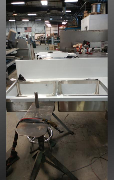
Welding and polishing are complete. The white peel coat covering remains to protect the main surfaces.
