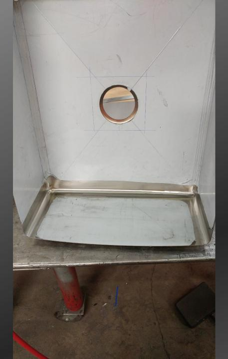
The welds are polished smooth. The bottom appears to be nearly seamless. The white peel coat protective covering remains.
