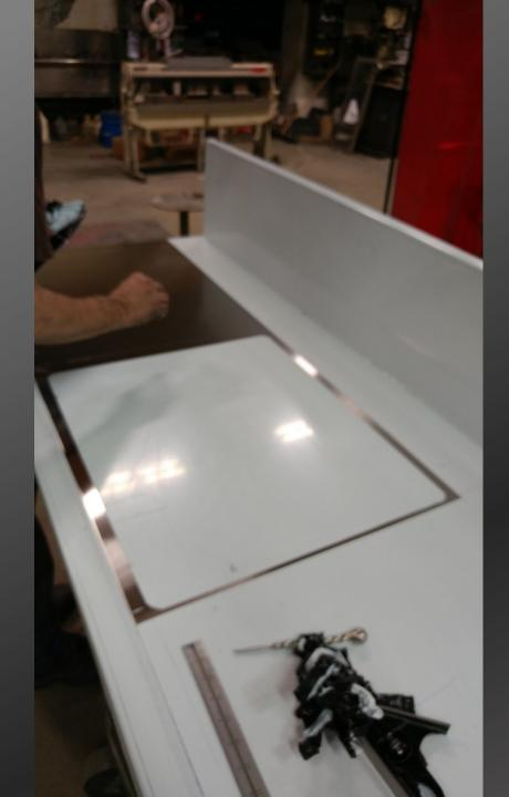
The backsplash and edges are formed. The countertop sink location are marked in preparation for cutting.
