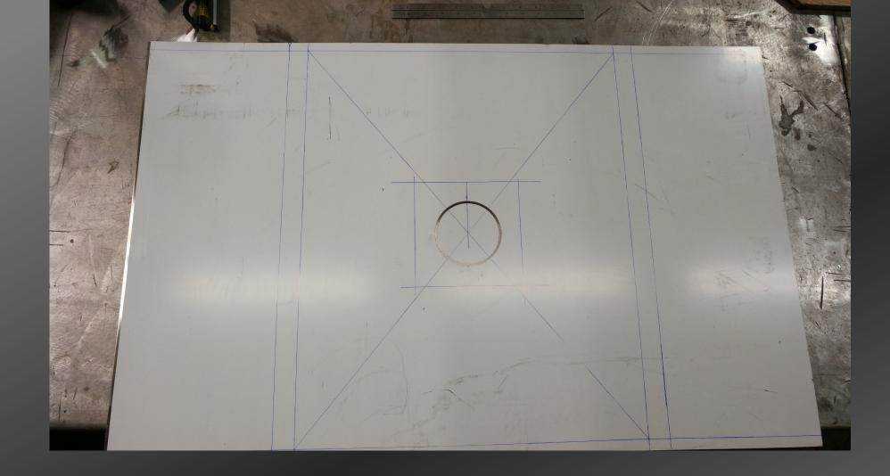
The sink layout is underway with blank piece of material and layout dimensions.
