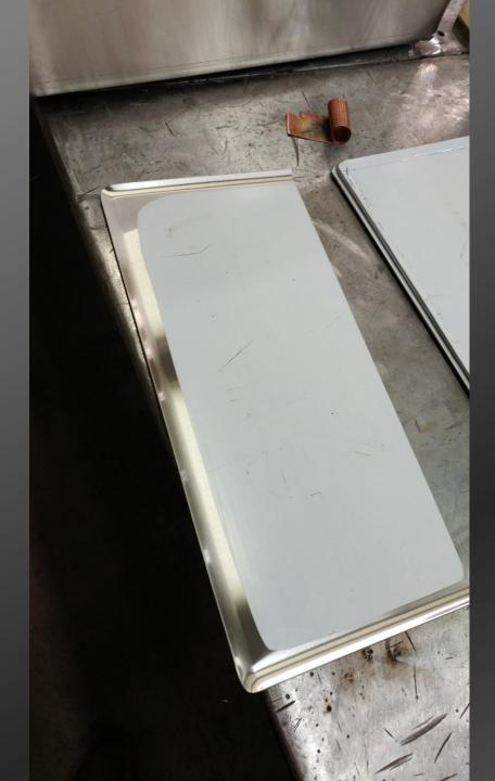
The opposite side pieces are formed and ready to be welded to the main sink blank
